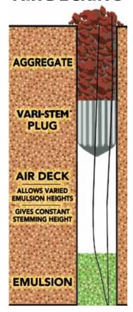
Besides reducing average rock diameter in the muck pile, **VARI-STEM**® Plugs save equipment and labor costs by reducing the quantity of oversized cap rock. It is possible to reduce stemming height using Vari-Stem, allowing more ANFO for greater cap rock breakage. **VARI-STEM**® and ANFO is cheap compared to secondary breakage costs (chemical vs. mechanical costs).
