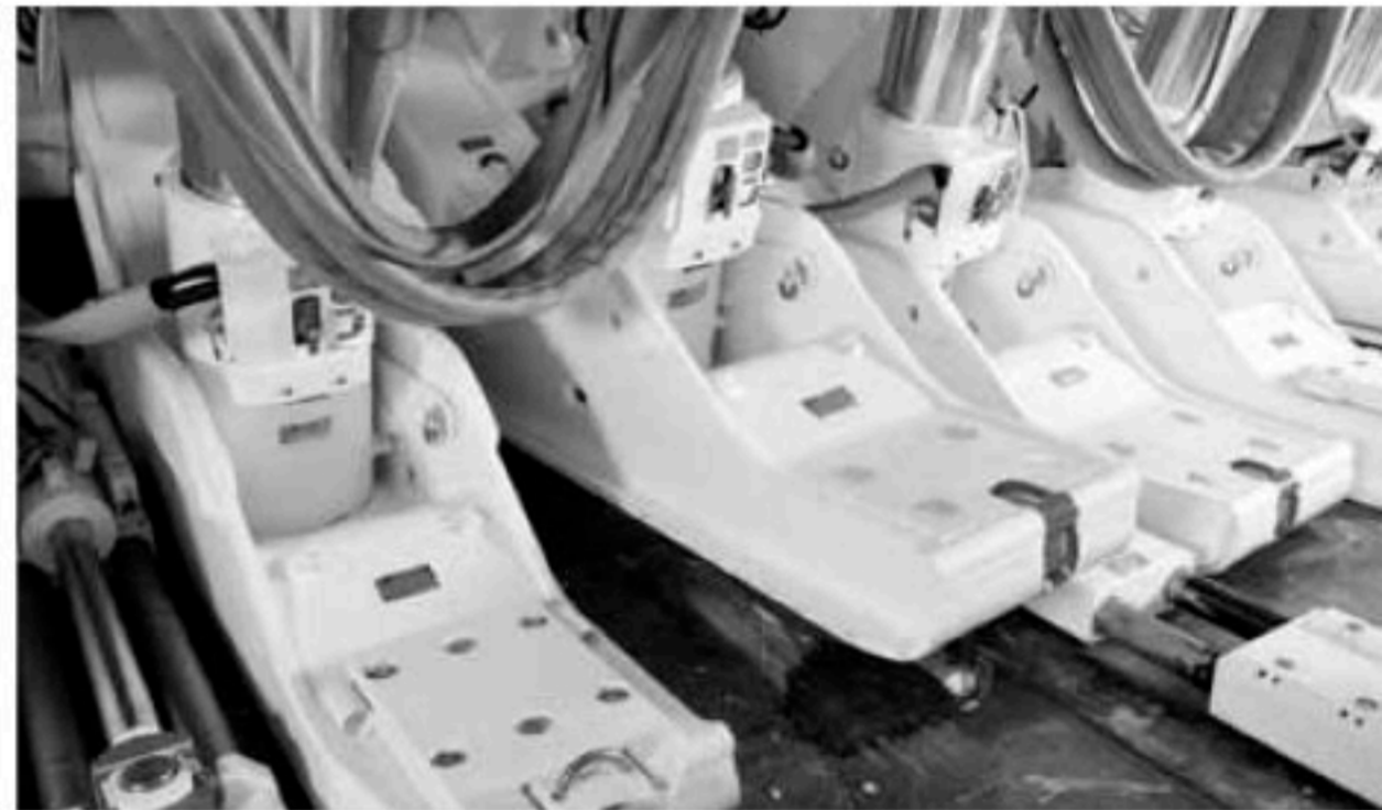
The elephant step (lifting one toe during advance)
