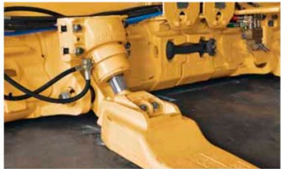
Horizon control for easy height adjustments
